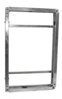
The Anti-Vibration mount is used to prevent vibration from the CHP from reaching the building, and to reduce the noise level cause by vibration. Installation is necessary when the unit is installed on a roof, indoors in an area with rooms/floors underneath or in certain basements.
